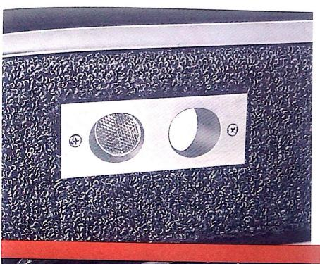
Thunderbird's luxurious door panel contains a courtesy light beamed toward the seat and a red warning light beamed toward the rear so traffic can see it from afar at night. This combined courtesy and safety feature is standard on the Landau and the convertible.
