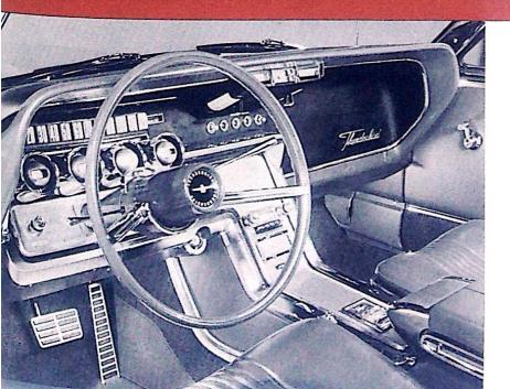
Like being in a cockpit. All controls and gauges are driver centered. A new instrument cluster features an easily readable row of floating gauges and a unique new drum speedometer with individually lighted numerals and a special lens which gives a thermometer-type indication of miles per hour.
