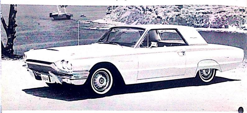
Longer hood, more sharply defined roof, smoother surfaces give Thunderbird a bullet-like shape that reduces wind resistance. This minimizes wind noise and cuts air drag which affects performance.
